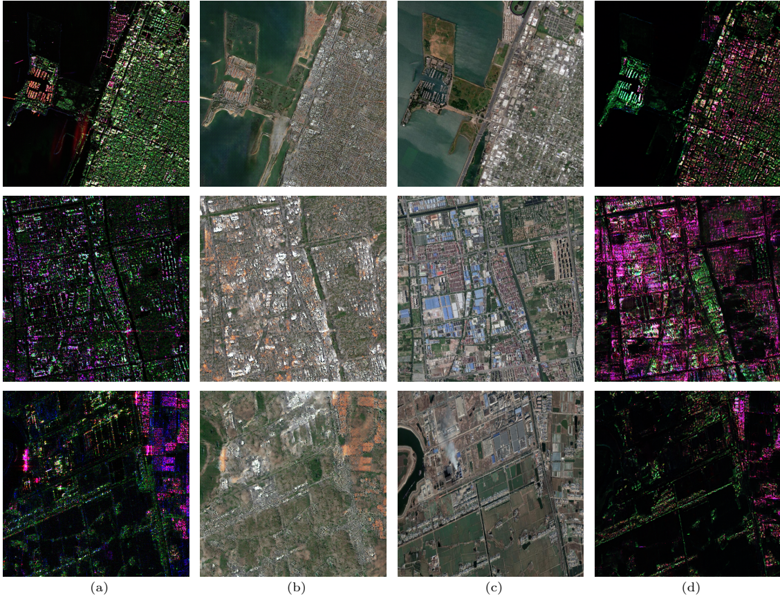
Figure S6 Images across scenes and across sensors reconstructed by the model pre-trained with 6 m UAVSAR images. Images in each row from left to right are (a) the real SAR image and (b) its translated optical image, (c) the real optical image and (d) its translated SAR image. Each row lists a kind of dataset: UAVSAR, GF-3 and ALOS-2.
