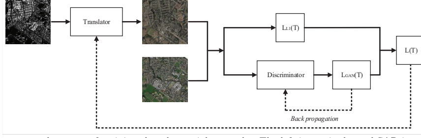
Figure S3 The conceptual process of training the adversarial networks. The left image is the real SAR image, the upper right is the synthesized optical image and the lower right is the real optical image.
